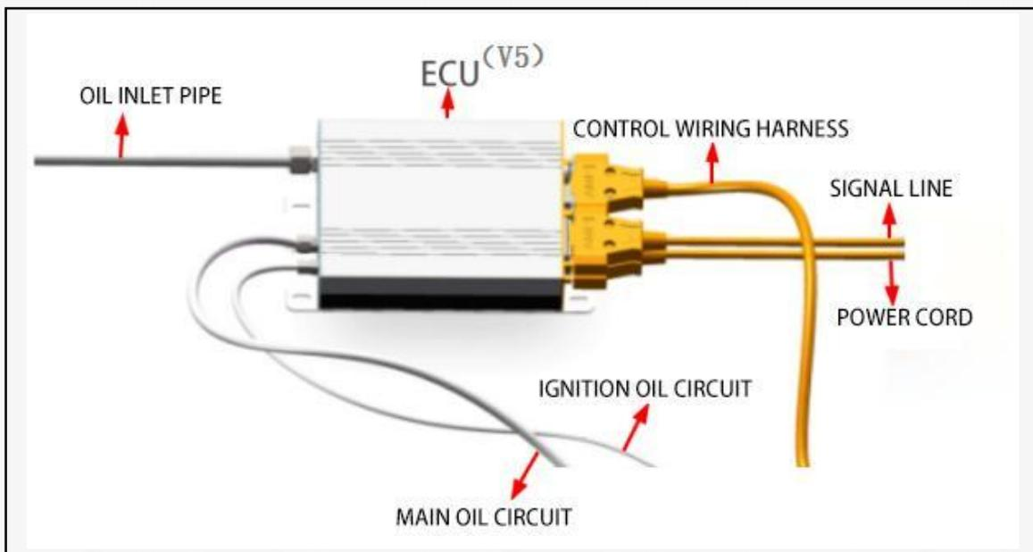
2. CONNECT THE ECU (V5) AND WIRING HARNESS AS SHOWN IN THE FOLLOWING FIGURE
