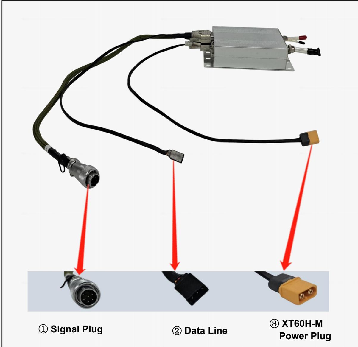
3. CONNECT THE ECU (V5) TO THE WIRING HARNESS AND ENGINE AS SHOWN IN THE FOLLOWING DIAGRAM
