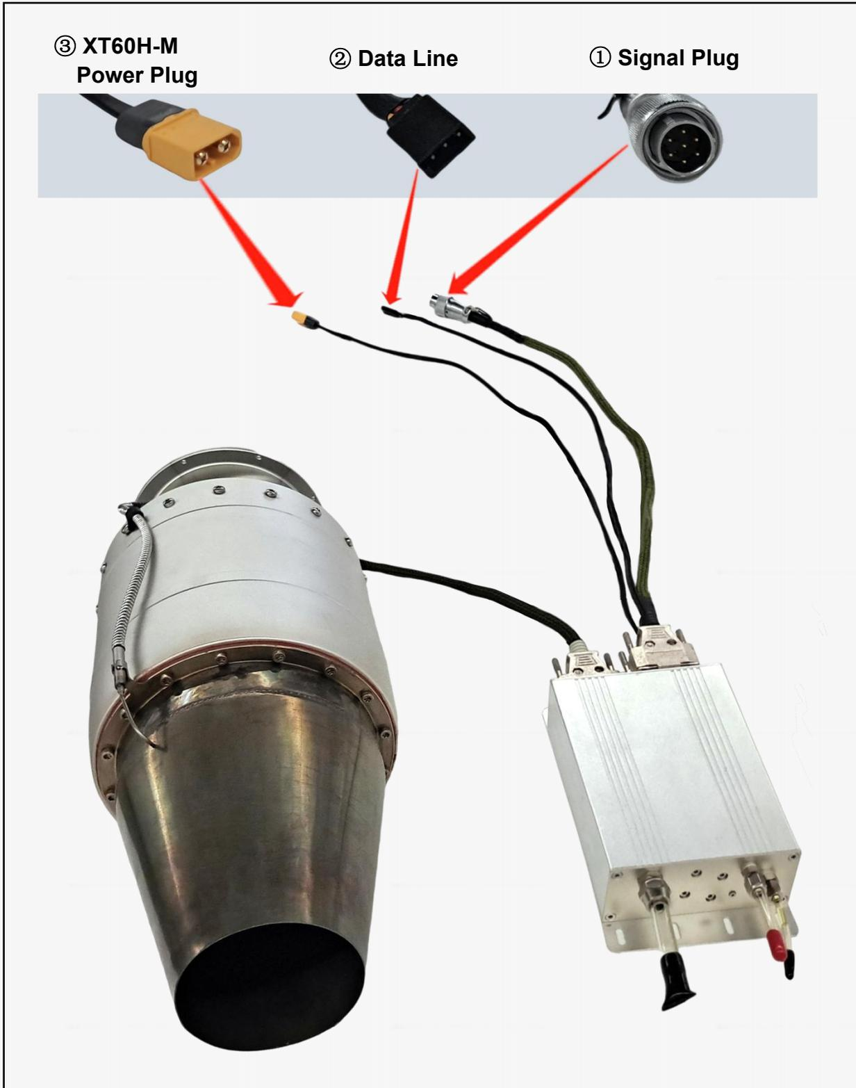
4.CONNECT AS SHOWN IN THE DIAGRAM BELOW, ECU (V5) IS CONNECTED TO THE COMPUTER THROUGH AN UPGRADE TOOL
