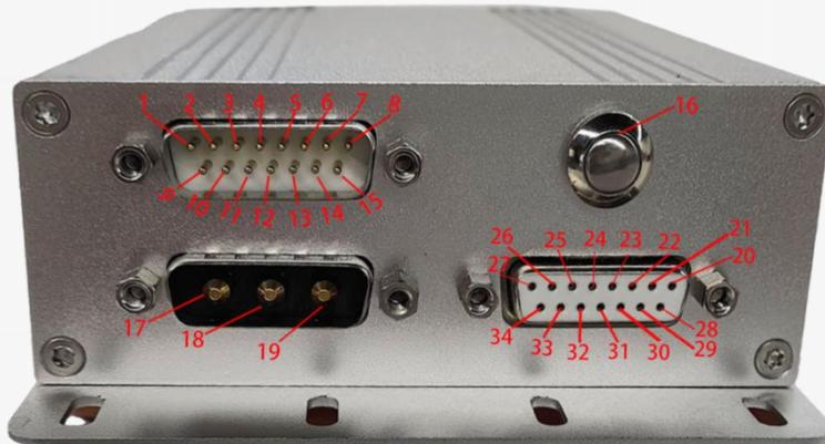
*pin 1-15 is an rs232/rs422 interface, used to connect external signal control devices and can be connected to rs232 or rs422 interfaces*
