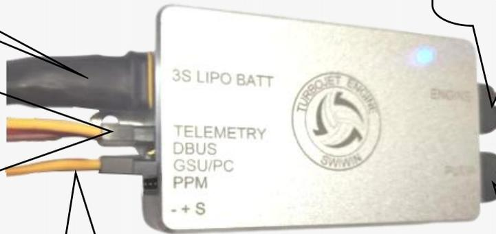
insert the equipped wiring harness here, and then connect the engine.
