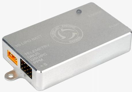
*ecu (v3) completes control of engine starting, acceleration and deceleration, steady state, and parking based on input control commands. under actual flight altitude, flight speed, and climate conditions, the ecu (v3) adjusts the fuel supply of the oil pump to maintain stable engine operation at a certain speed.*
